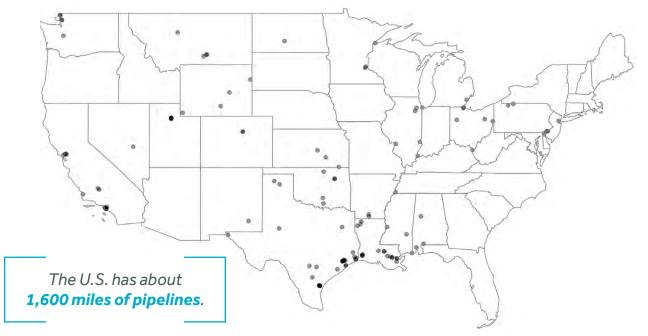
Currently, of the world's 2,900 miles of dedicated transport pipelines for hydrogen, the United States has about 1,600 miles of pipelines with much of the infrastructure along the Gulf Coast near refineries.<sup>27</sup> Other notable U.S. hydrogen infrastructure includes the world's largest storage facility in Texas where hydrogen is stored in underground salt caverns.<sup>28</sup>
